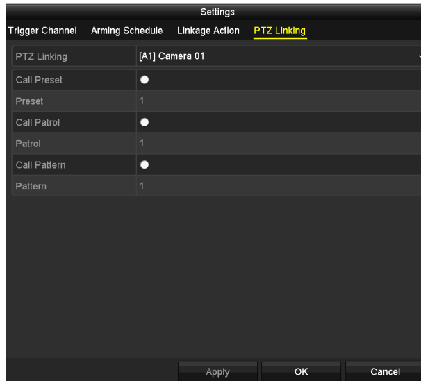
Figure 8-7 Set PTZ Linking of Alarm Input
